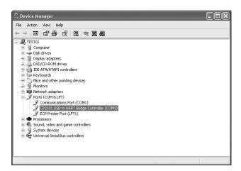
**USB-RS232 Convertor** will usually use the lowest available COM port for operation. For instance, if COM ports 1 to 3 are in use by other peripherals and applications, **USB-RS232 Convertor** will use COM 4.
